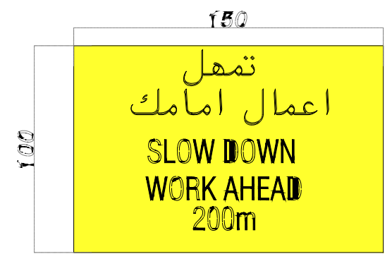
WORK AHEAD SIGN PROVIDED AT 500m AND 100m LEFT AND RIGHT
