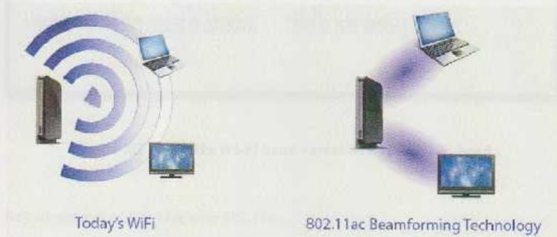
Figure 2.1 : Today's Wi-Fi versus Beamforming Technology
