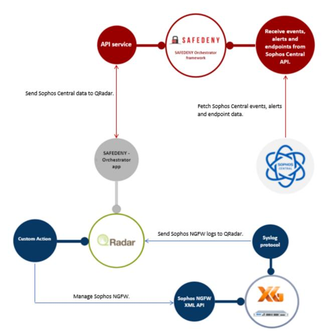
Figure 3.3: Integration framework diagram.
