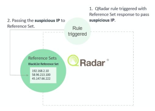
Figure 3.1: Reference set as a rule response diagram.
