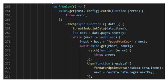
Figure 4.4: Part of fetch endpoints data function.
