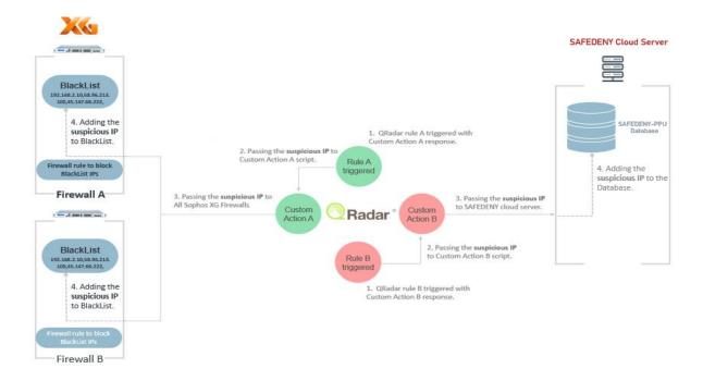
Figure 3.2: QRadar Custom Actions diagram for passing suspicious IP to Sophos NGFW and database.
