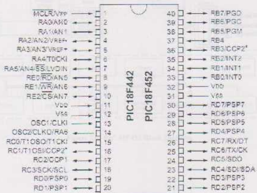
Figure 2.8: Pins of PIC 18F452 Microcontroller
