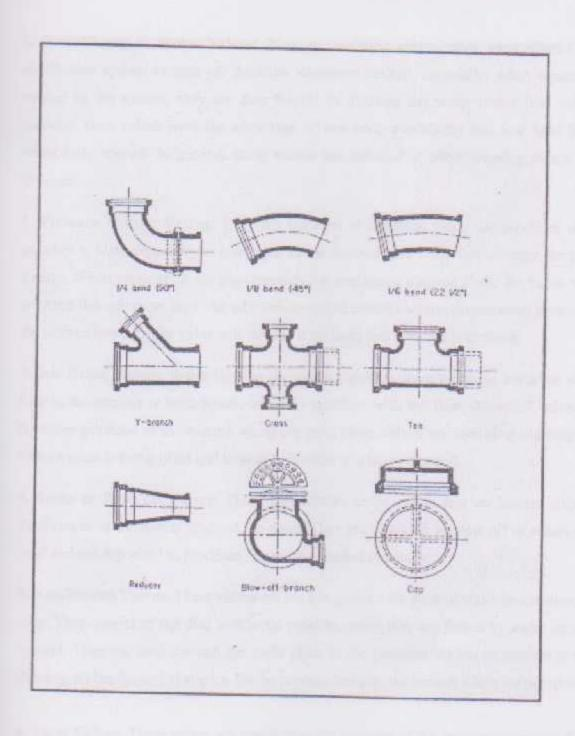
Figure 3.1: Various Pipe Fitting
