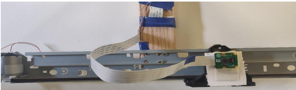
A wooden item that carries the printer rail which holds the camera.
