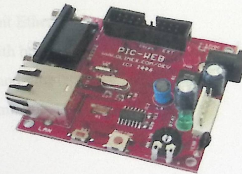
Figure 3-2 PIC web server with PIC18f452 and enc28j6
