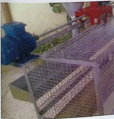
Figure 5. 15: Hopper with motor and the feeder
