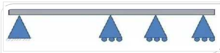
Picture 27: continuous beam
