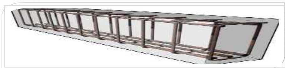
Picture 28: Reinforced concrete beam
