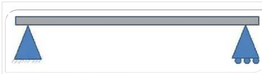
Picture 24: simply supported beam
