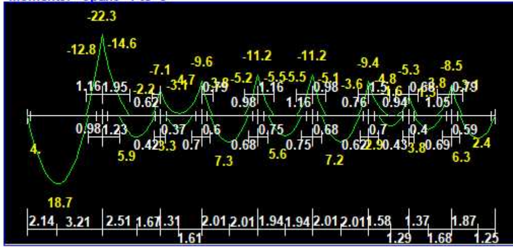
Picture 48: Moment envelope of Rib
