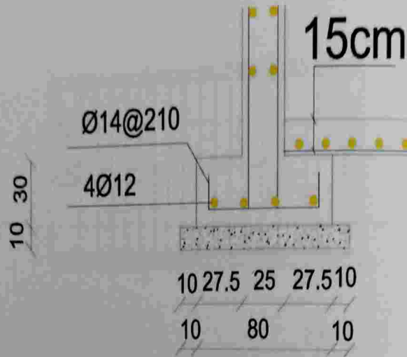
Figure (4-24) Strip Footing Detail
