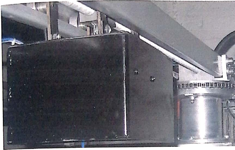
Figure (7.2): Practical power screw-mechanism of trolley translation.
