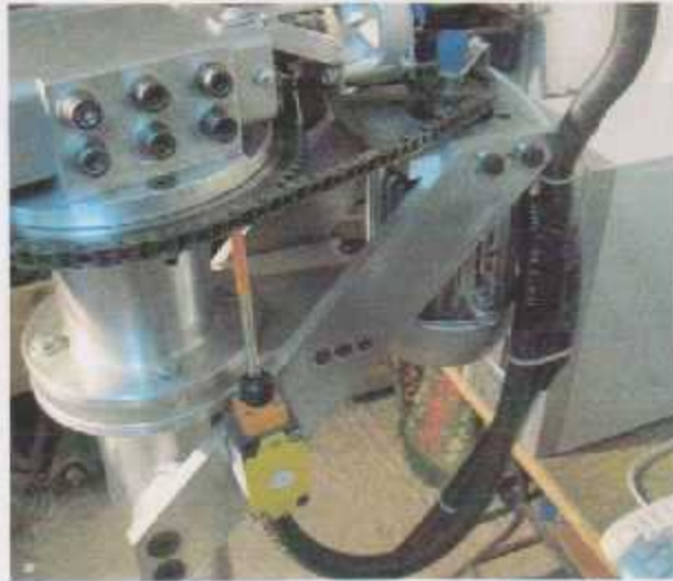
Figure (7.1): Practical rotation motor mount.
