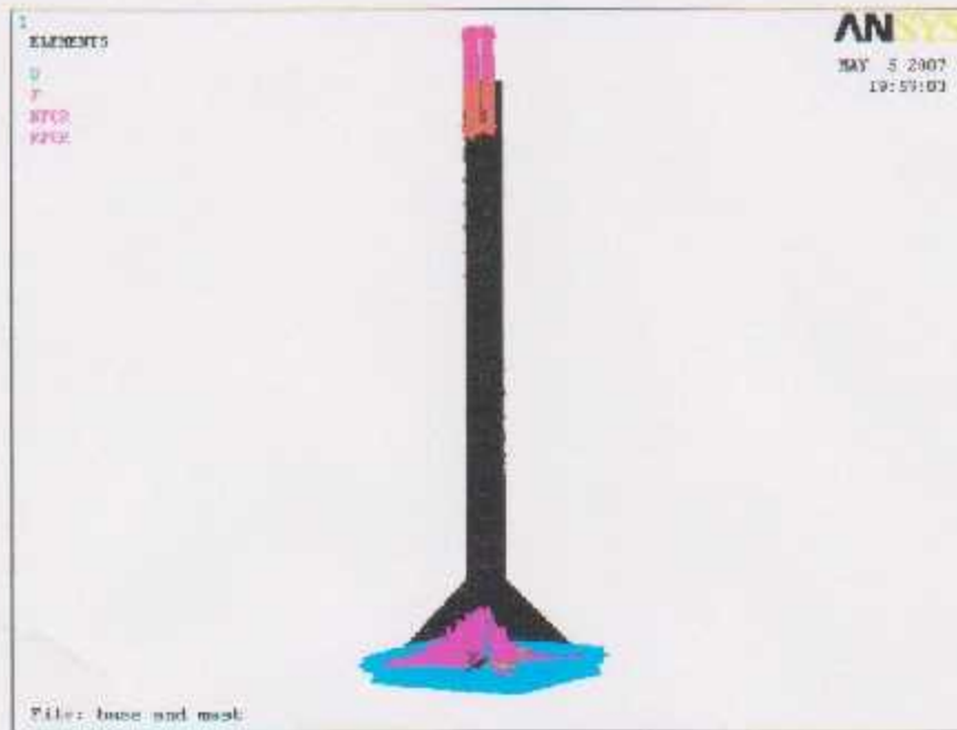
Figure (4.13): Load distribution among the mast.
