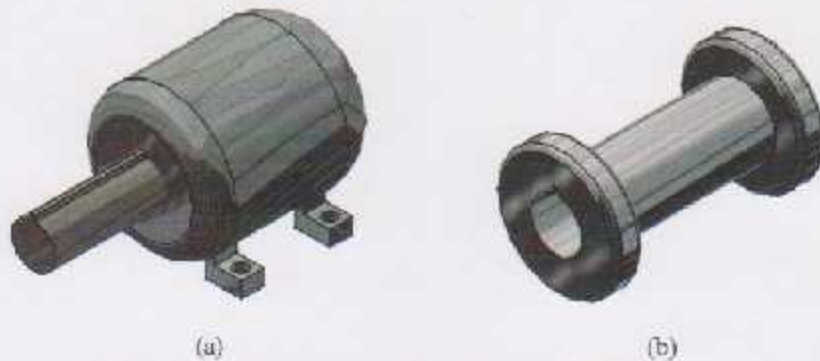
Figure (2.3): Trolley parts: (a) Hoisting motor, (b) Pulley.
