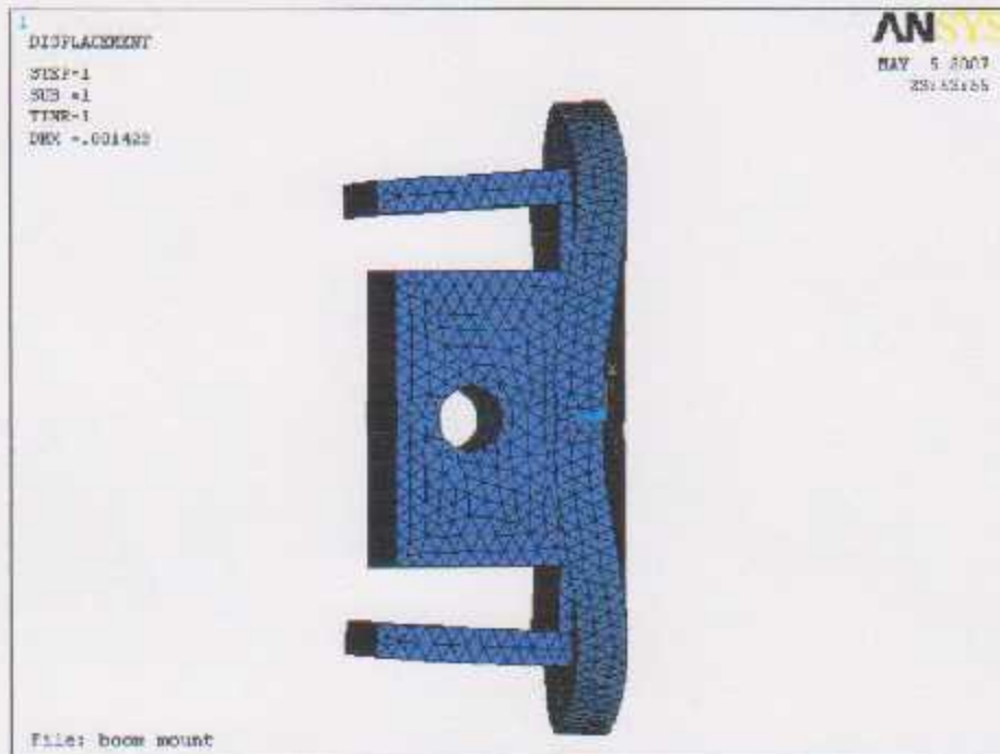
Figure (4.7): Deformations in the boom mount.
