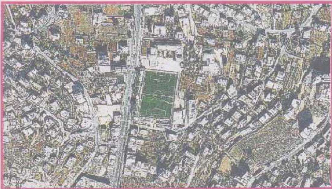
Figure (6.30) Sample of 2006 image after applying 3*3 high pass filter
