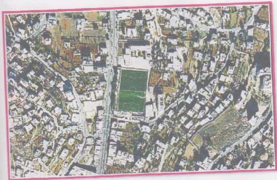
Figure (6.32) Sample of 2006 image after applying 7*7 edge enhancement filter
