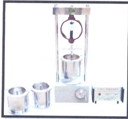
Fig 5.28 the penetration device
