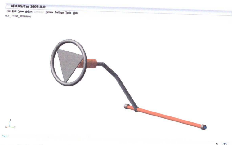
Figure 2.1- The steering subsystem from ADAMS/Car software.[9]
