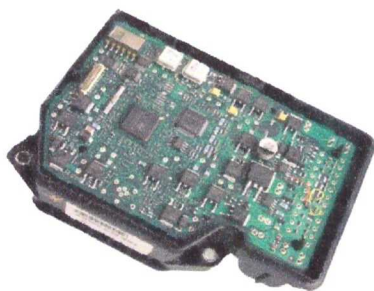
Figure 5.25- Slip Control System ECU with Integrated Inertial Sensors.
