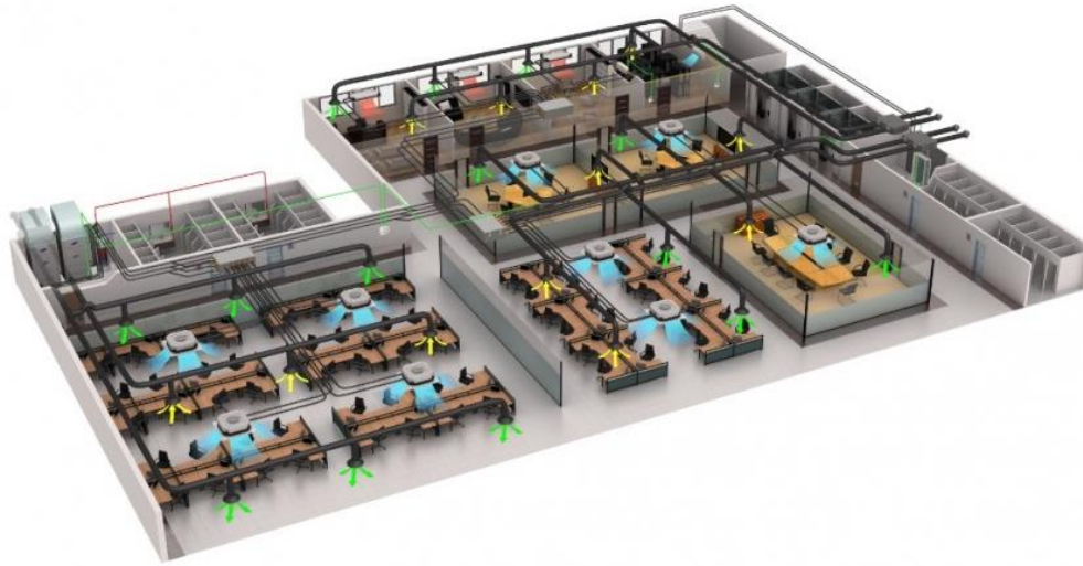
Figure (3.6): Water cooled type VRF system
