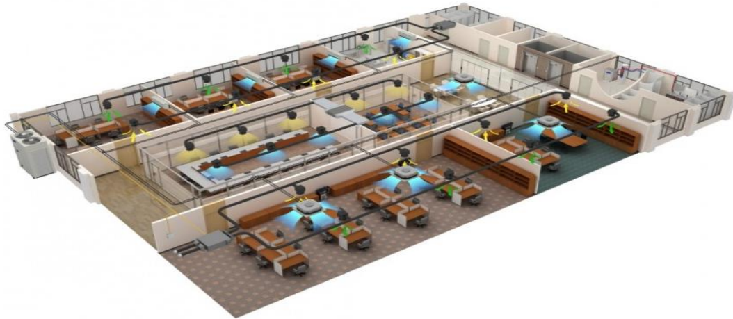
Figure (3.4): Heat pumps type VRF system
