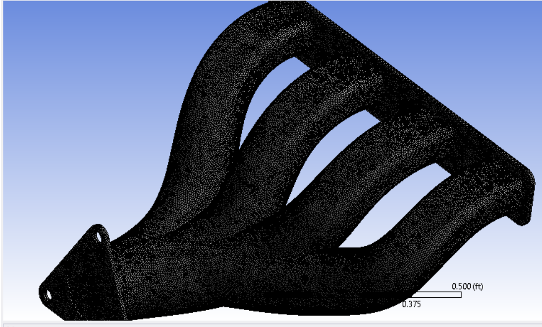
Figure 4.17 Mesh update in Fluid Flow application
