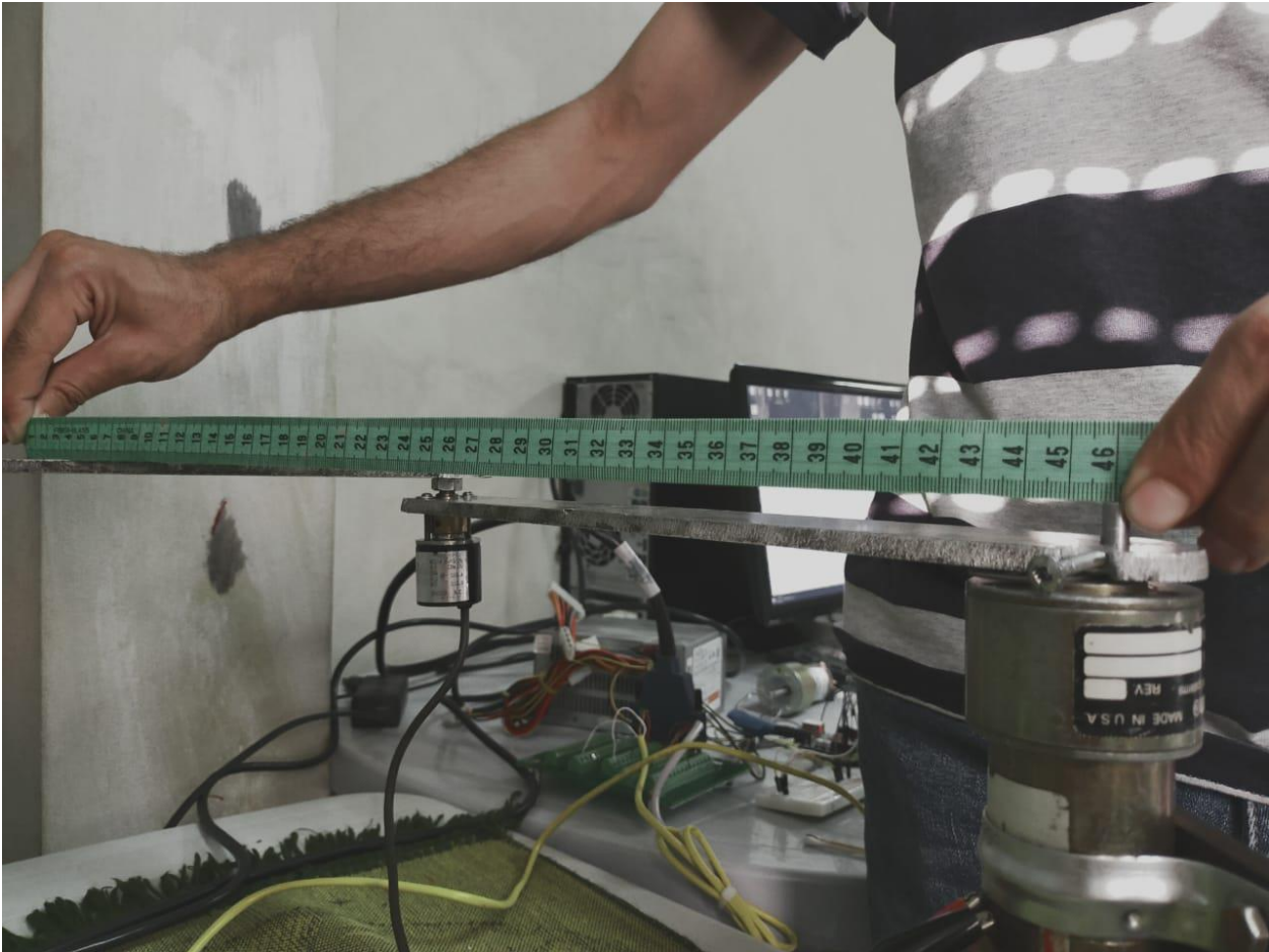
Figure 5.48: Measurement of the radius at desired radius=45cm
