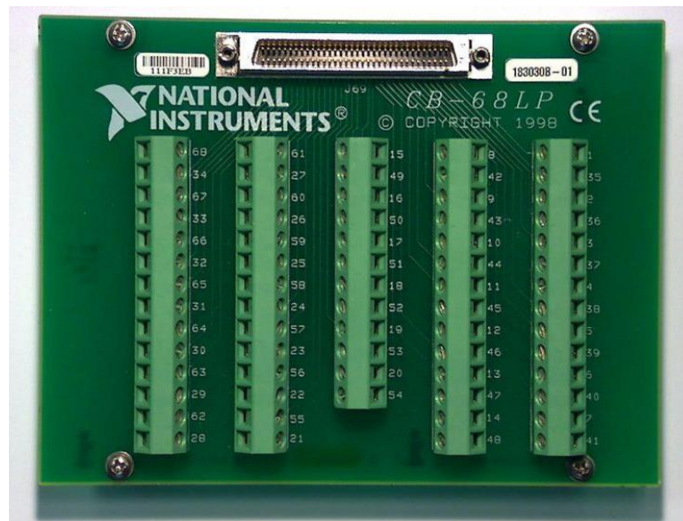
Figure 3.15: NI-6221 screw terminal connector
