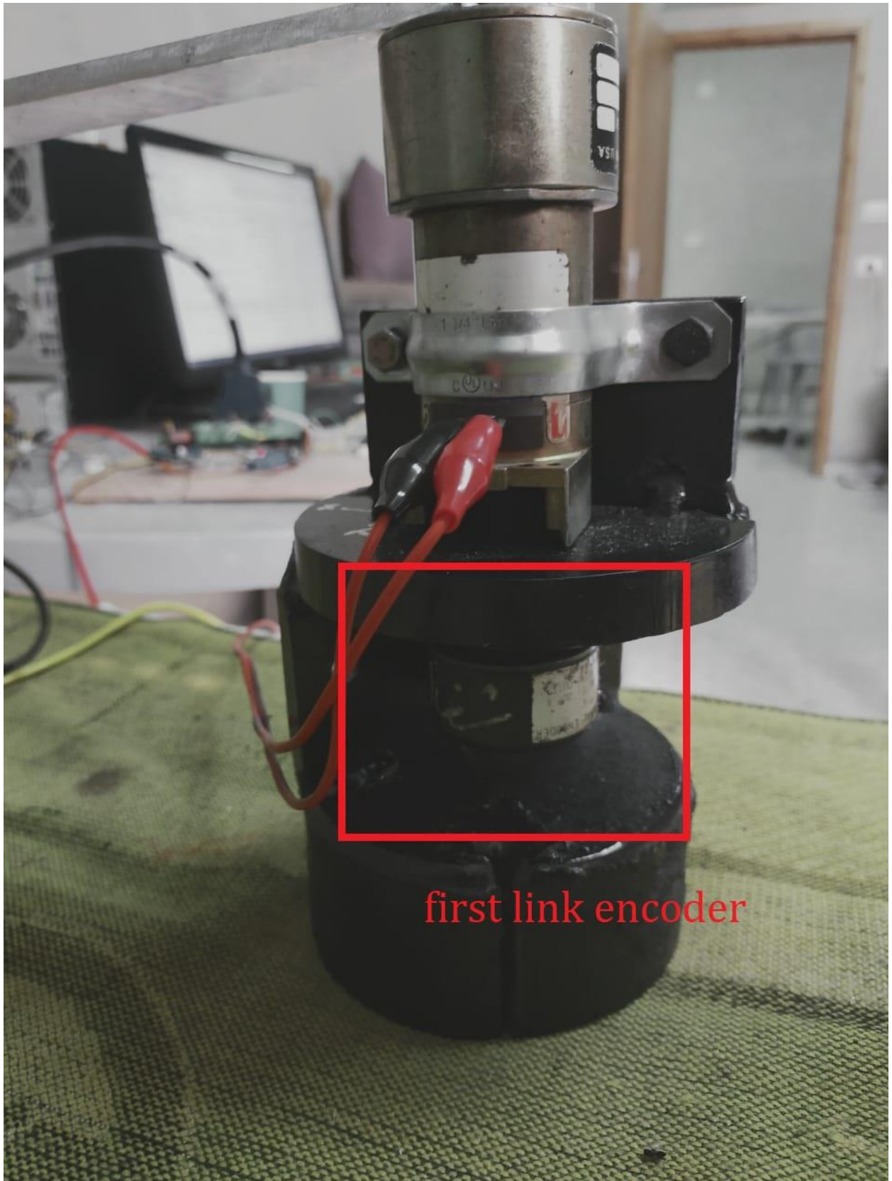
Figure 3.21: First link encoder in the project
