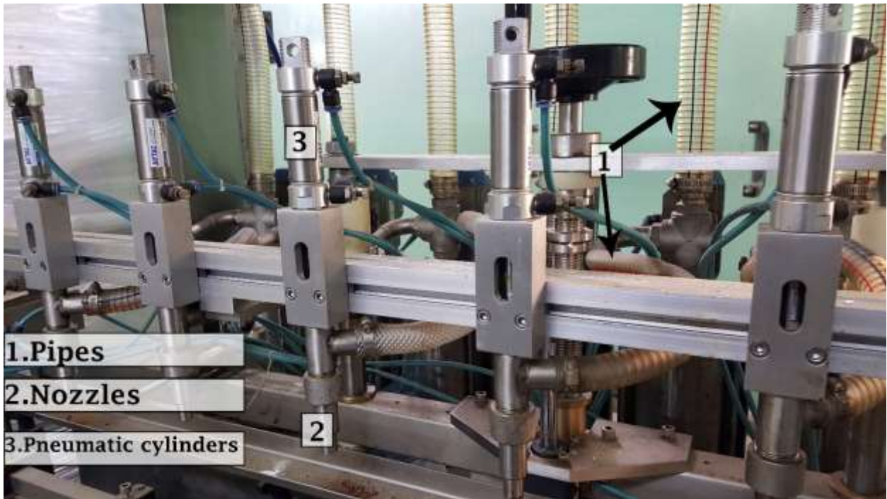
Figure 1.6 Pipes, nozzles and pneumatic cylinders.
