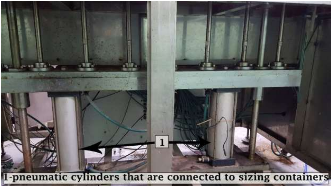
Figure 1.7 Pneumatic cylinders that are connected to sizing containers.
