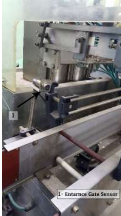
Figure 1.4 Entrance gate sensor.
