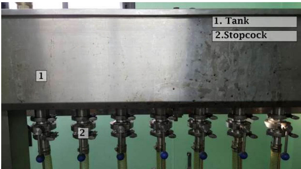
Figure 1.2 Tank and stopcock.
