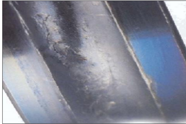
Figure 4 Lubricant failure bearing
