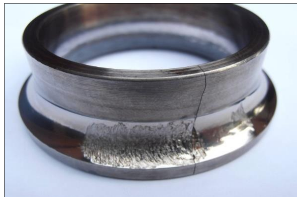
Figure 2 Excessive load bearing
