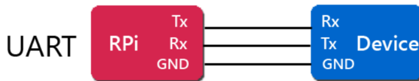
Figure 6. 5 : RPi-UART port connected to a device [13]
