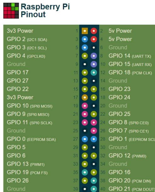
Figure 6. 3: GPIO pins for Raspberry Pi 4 – model B
