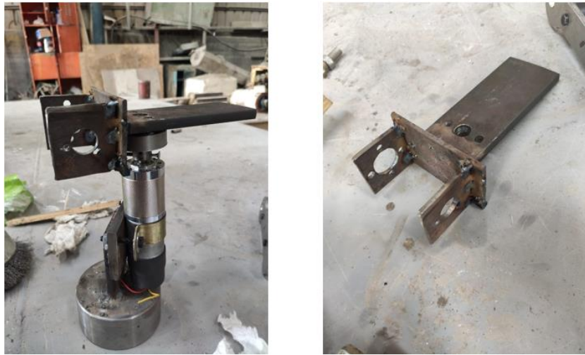
Figure 8. 1: The base of Excavator manipulator.
