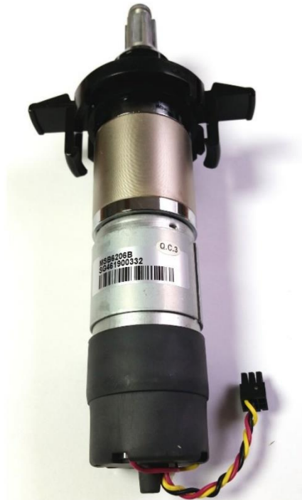
Figure 5. 4: The selected DC brush motor for joints 1 and 2
