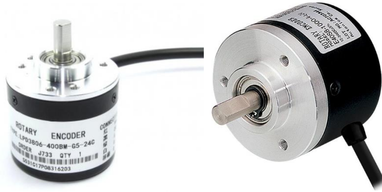
Figure 5. 10: The used rotary encoders: 400-pulse resolution (left), 2048-pulse resolution (right)
