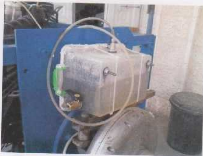
Figure (4-1) the practical hydrogen extraction device as we built ready to be connected with power source.
