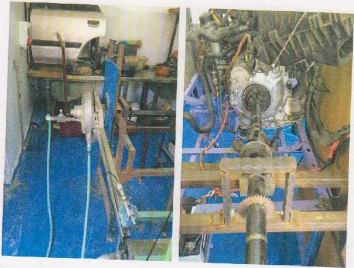
Figure 6.8 The dynamometer (Water brake absorber)
