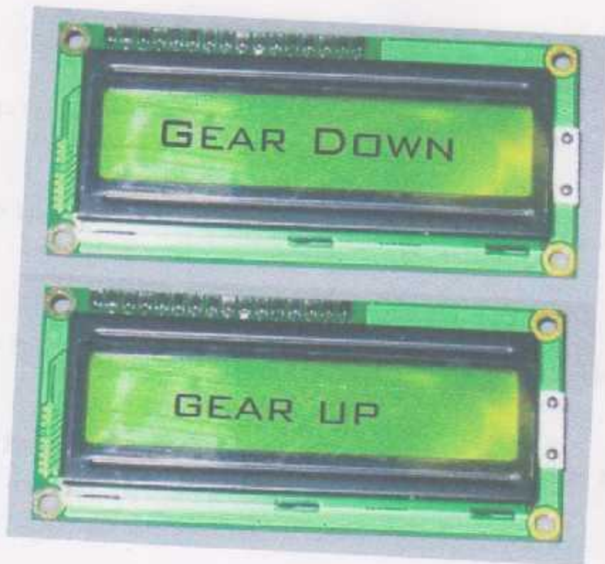
Figure (5-2) LCD to warn driver to shift up or shift down gear ratio
