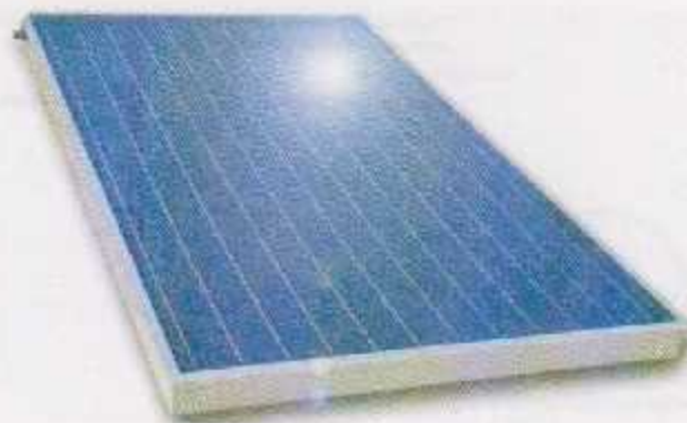
Figure (3.7): Flat plate collector with selective coating on the absorber. The parallel lines indicate where the riser tubes are connected to the absorber by ultrasonic welding.
