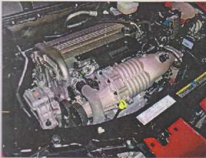
Figure (2-2) shows a screw supercharger and its location on the car engine
