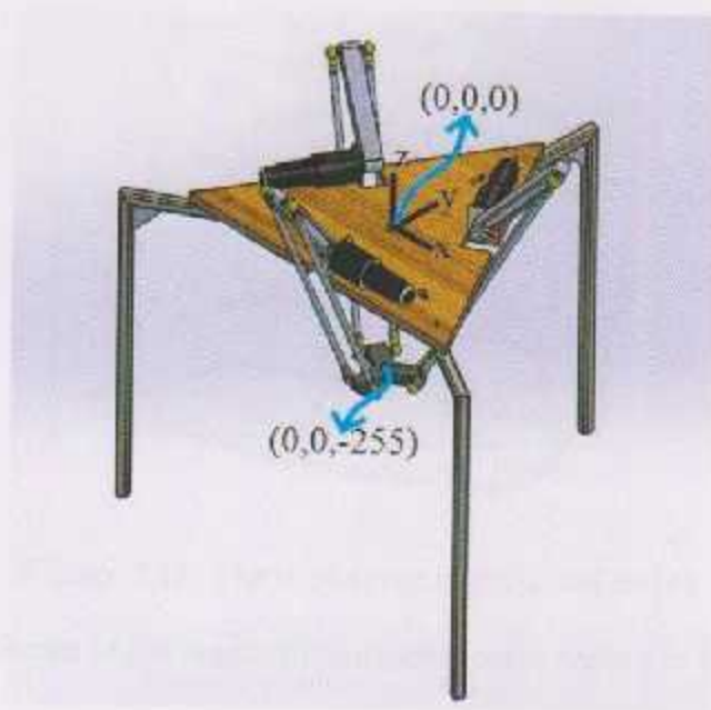
Figure 7.9: Minimum distance along z-axis.
