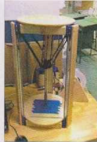
Figure 2.3: (a) Rostock (delta robot 3D printer), (b) Customized MOST Delta RepRap.
