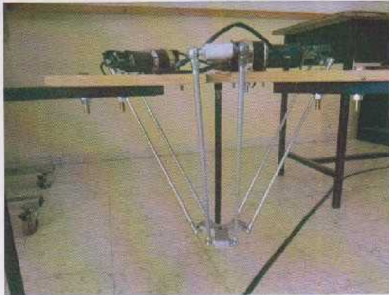
Figure 7.4 : The mechanical parts of delta robot be assembled with the actuators.
