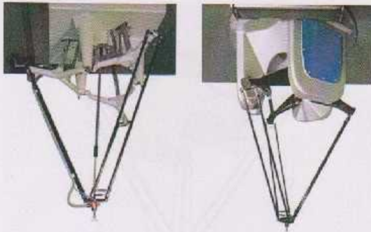
Figure 2.5: Two of the three Delta robot models offered by SIG Pack Systems, C33 and CE33.
