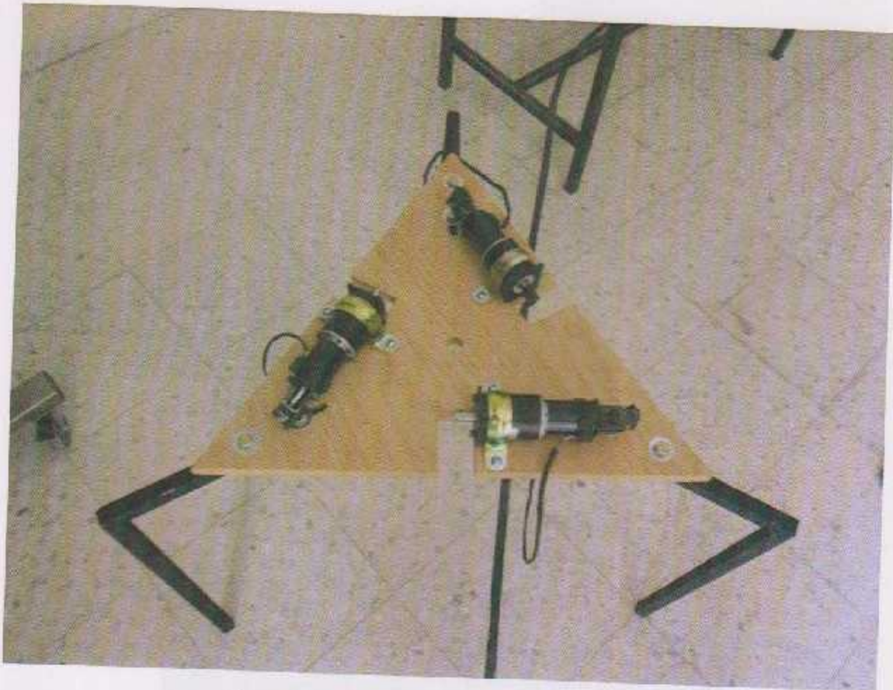
Figure 7.2: The actuators are fixed on the base.
