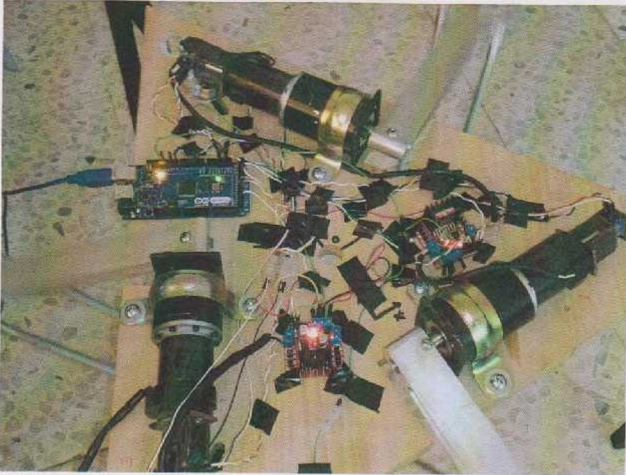
Figure 7.5: The connection of the microcontroller and drivers with the actuators and encoders.
