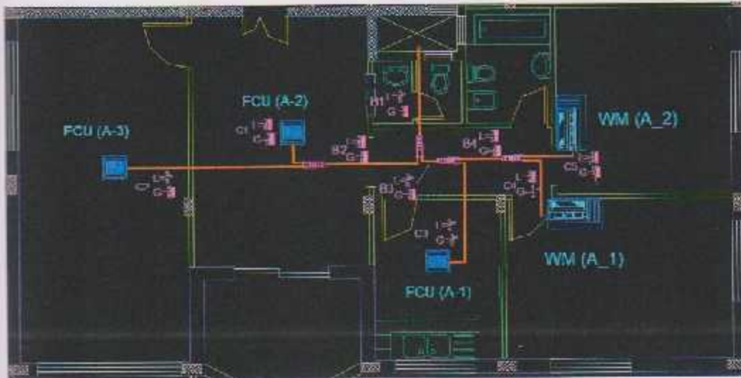
Figure (5.10): Indoor units' distribution.
