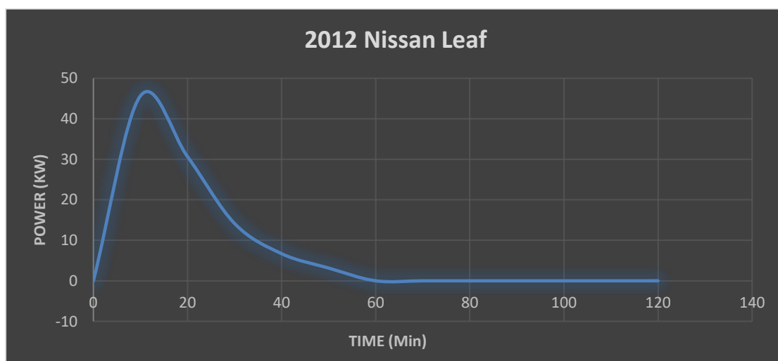
Figure 4.14: A DC fast charge is shown for a 2012 Nissan Leaf charged with a 50KW [36].
