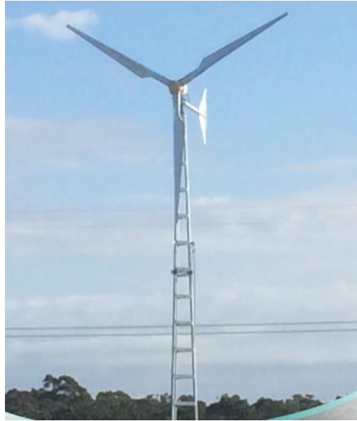
Figure 4. 8: AWS5.1kW wind turbine.
