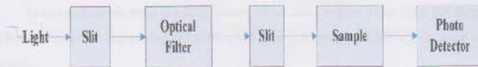
Fig (3.6): light path block diagram
