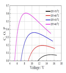
Figure 3.2: (Standard Performance Graph COP = f(V) of  $\Delta T$  ranged from 40 to 60/70 °C)
