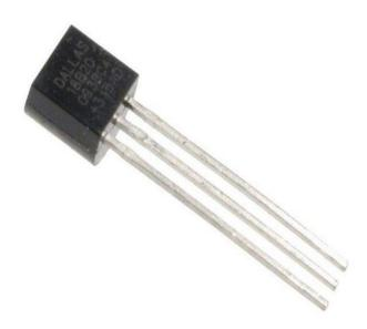
Figure 2.8: Temperature Sensor (Im35).
