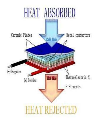
Figure 1.1: working principle of TEC module.
