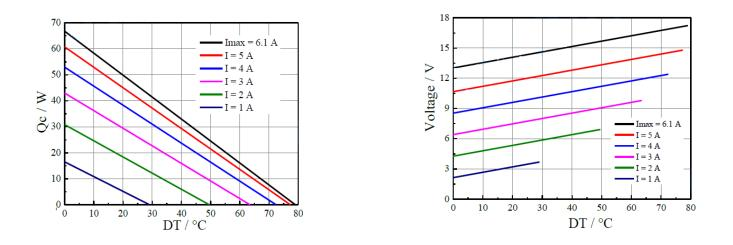
Figure 3.1: TEC Module Performance Graph (Obtained From TEC Module Spec Sheet)
