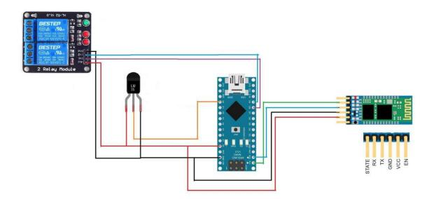
Figure (4.3): Electric circuit control temperature.
