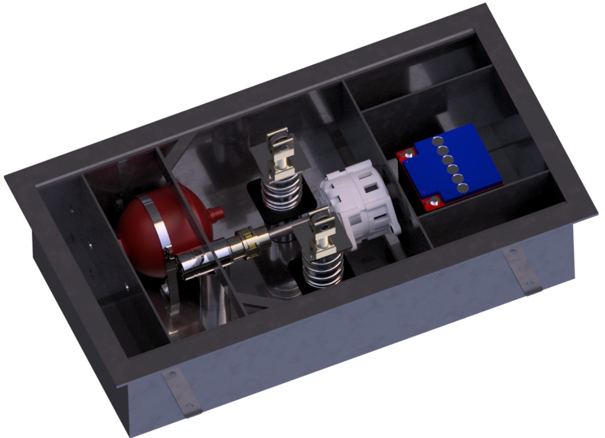
Figure 3.1: unit Selected for power generation using hydraulic speed bump mechanism
