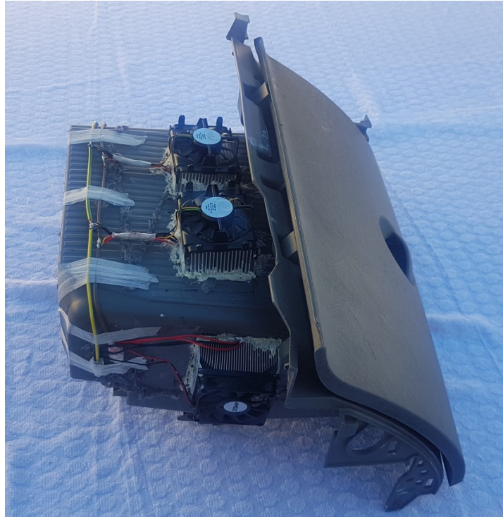
Figure 3.4: Schematic diagram of glove thermoelectric refrigerator cabinet (1) outer casing (2) Peltier Module (3) Heat sink (4) insulation sheet
