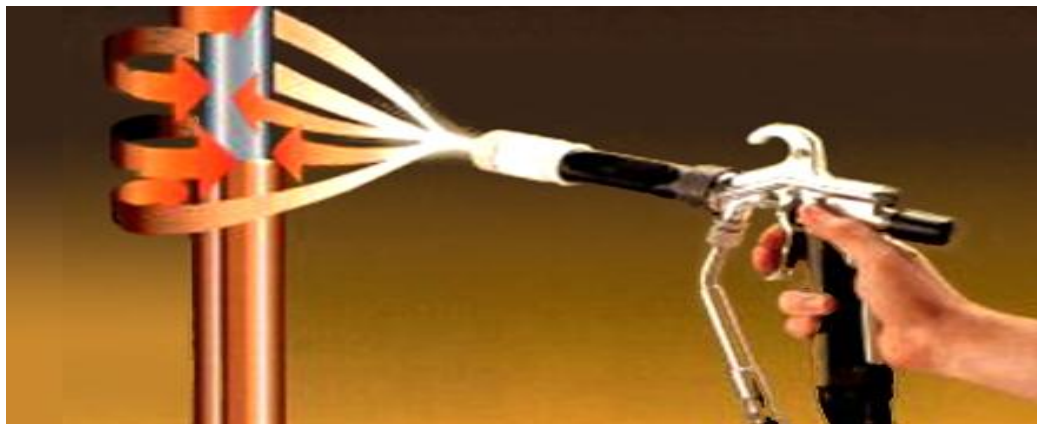
Figure 2: Paint using ionized paint grains.
