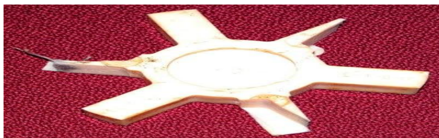
Figure 3.6: Wear due to misalignment 1.
