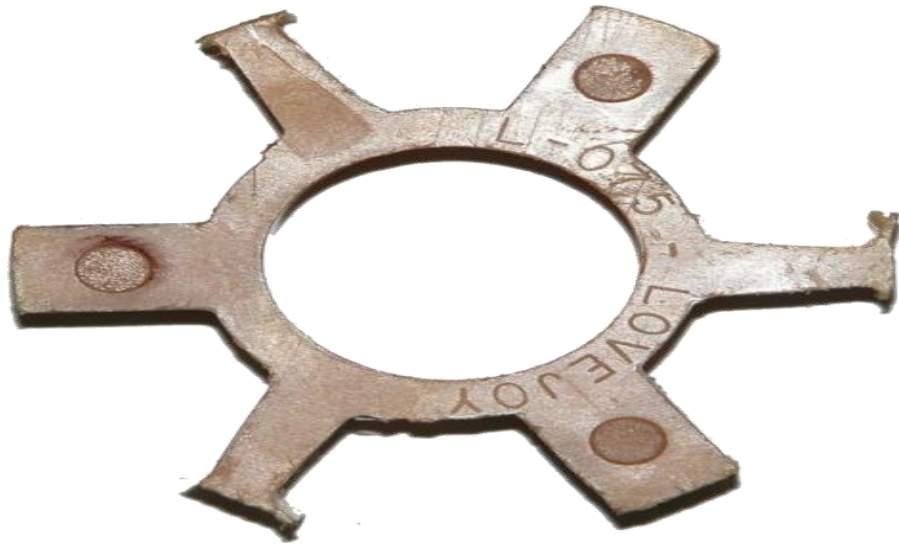
Figure 3.4: Normal wear similar on all contact point.
