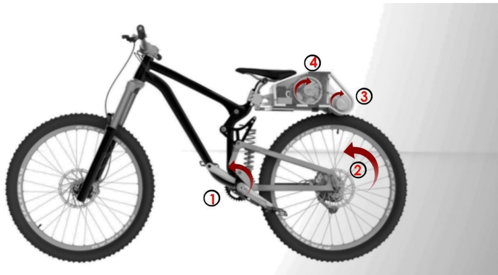
Figure 2.6: The steps to transfer rotational force from paddle to generator.
