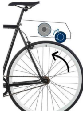
Figure 2.18: Wheel torque transferred to roller
