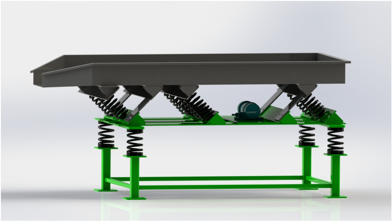
Figure 3.4: Grape Fruit vibration Table Feeding the Convyer
