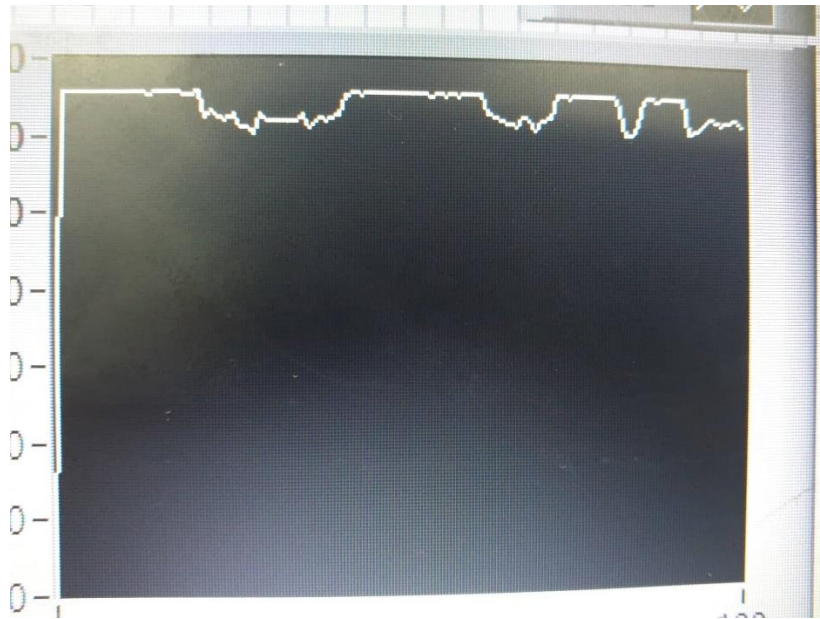
Fig5.3: output of detector1 when darkness
