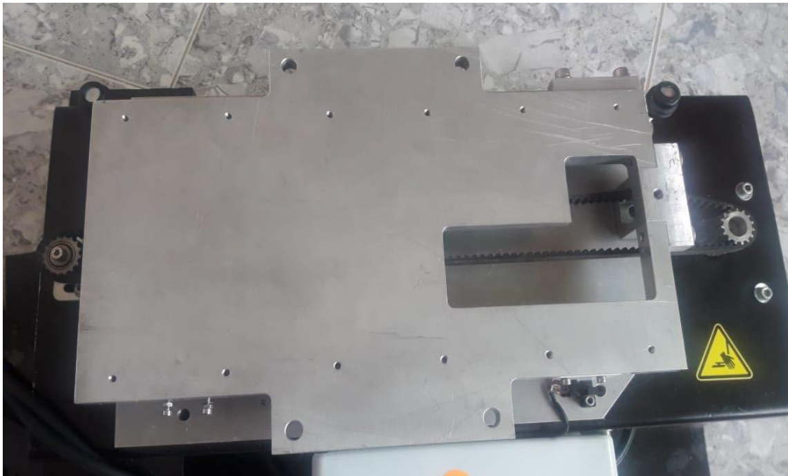
Figure3.5: Timing belt and two gear mechanism.
