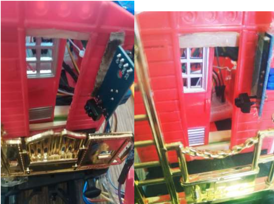
Figure 4. 1 : Test Infrared sensor (IN door , OUT door )
