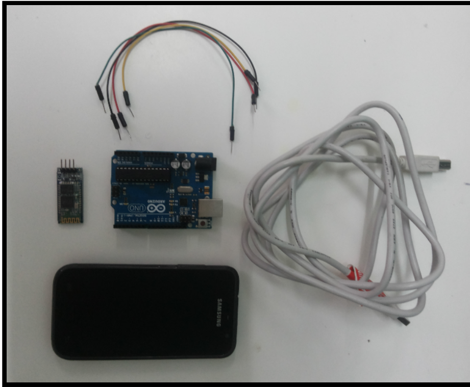
Figure 6.1: Electrical subsystem components
