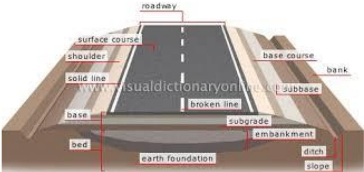
شكل 7-19: typical cross section ditch
