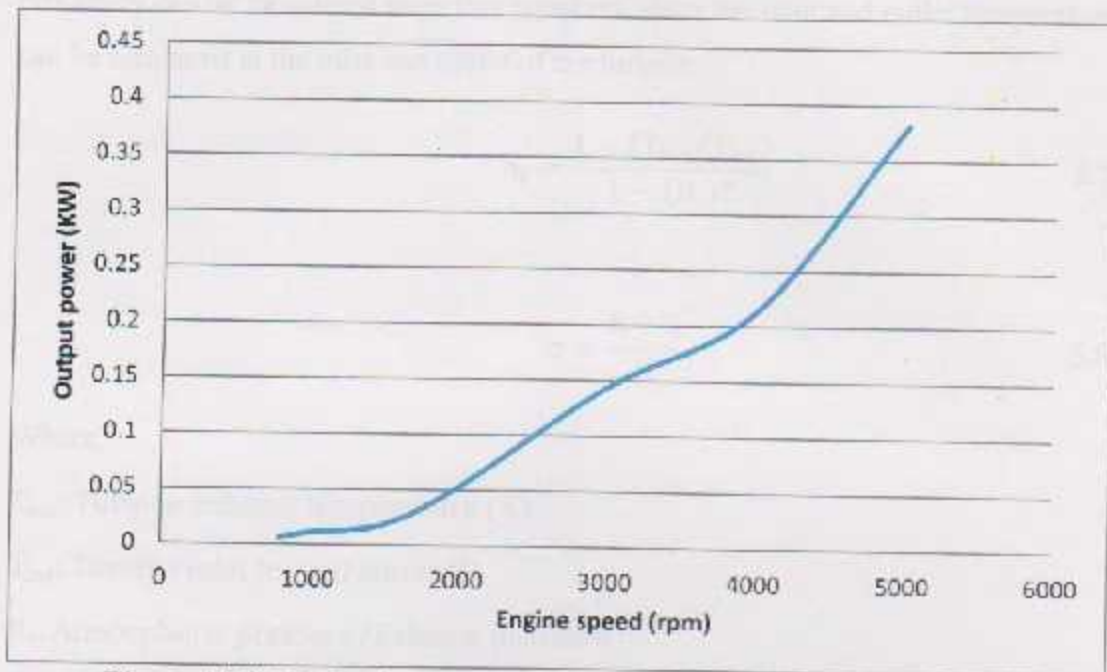
Figure (5.3) Relation between engine speed and turbine output power
