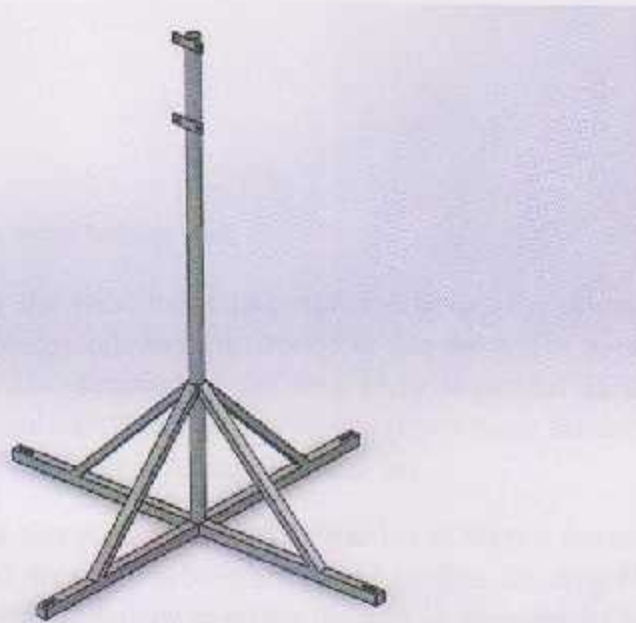
Figure 4.10- Turbine Steel tower
