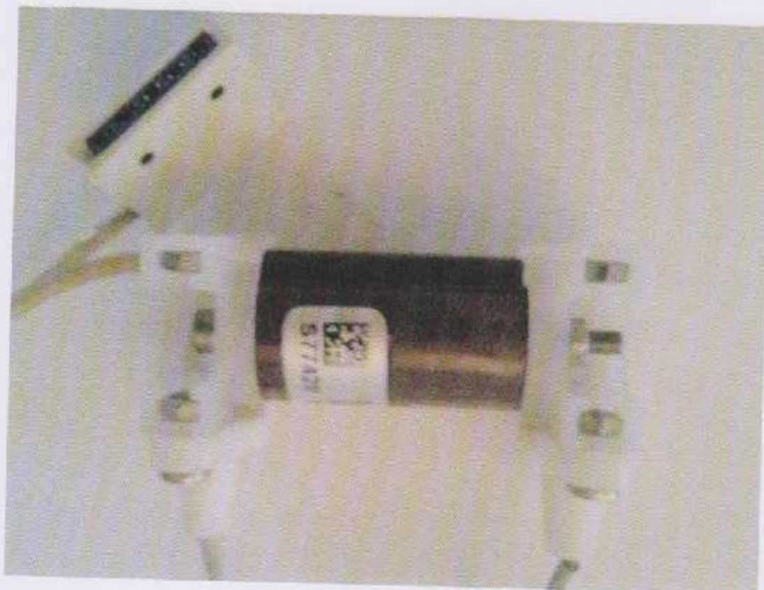
Figure 6.1: 3-poles conductivity cell.
