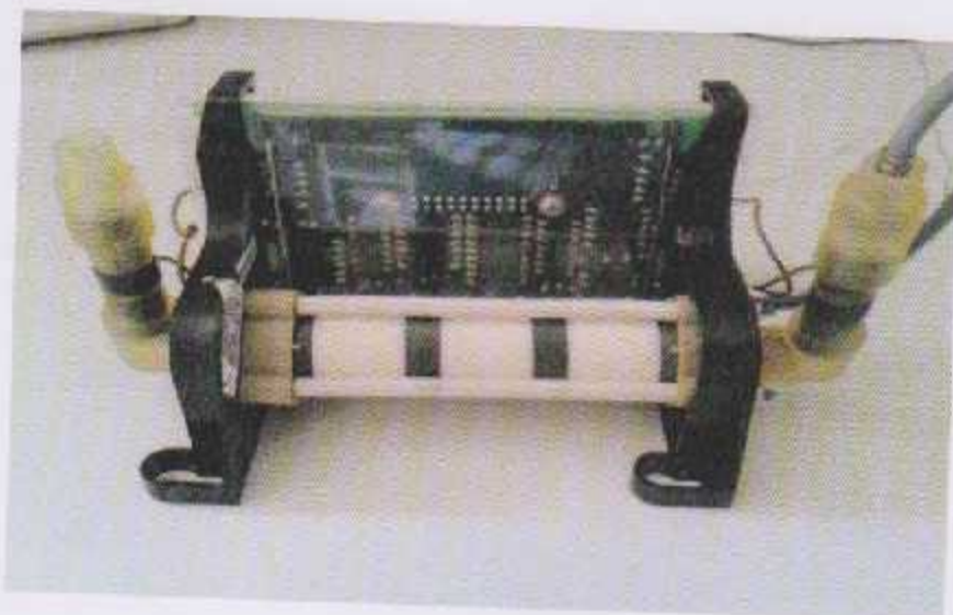
Figure 6.2: 4-poles conductivity cell
