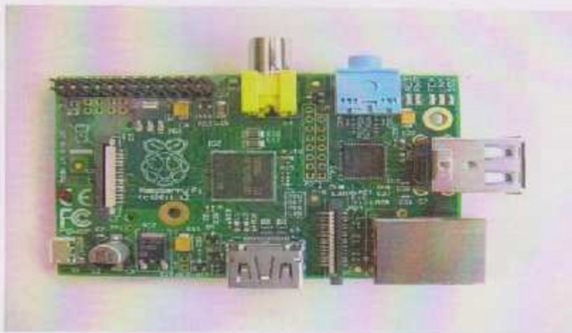
Figure 2.16: Raspberry pi Model B+
