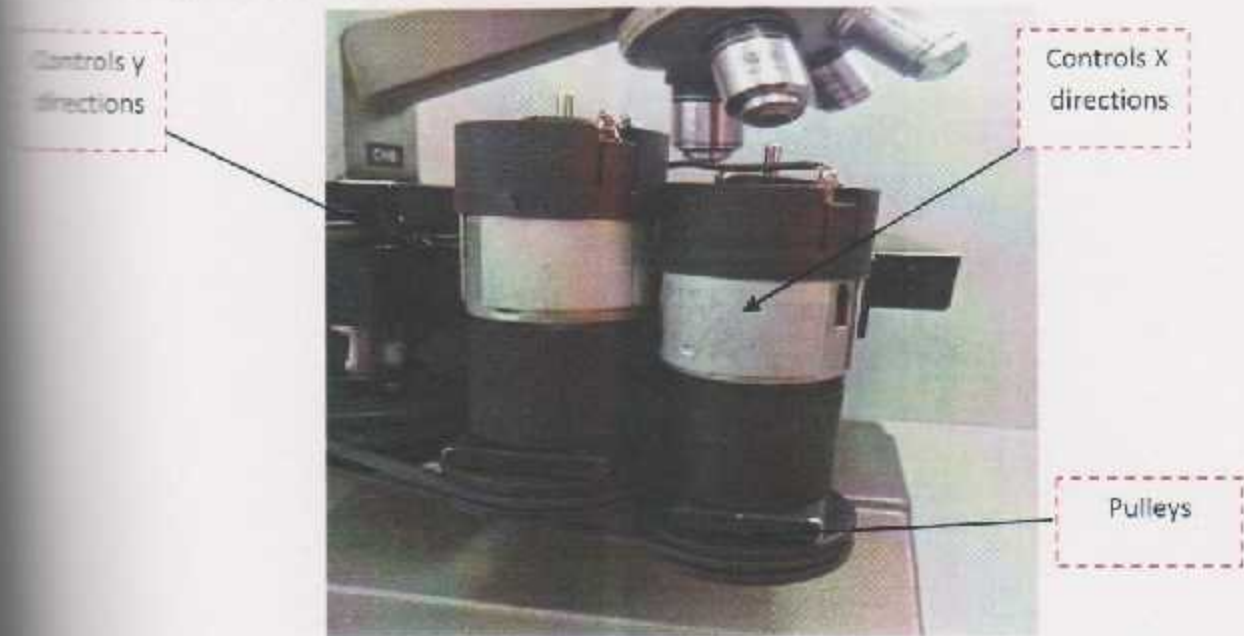
Figure 5.4: Attaching Gear DC-Motors to Microscope knobs for XY direction
