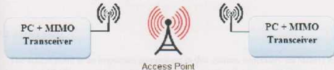
Figure 4.11 :Block Diagram of MIMO Wi-Fi Devices Connection
