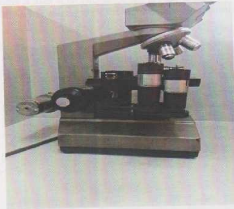
Figure 5.3: DC-Motors Fixed in the Microscope Stage
