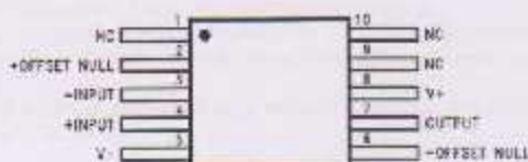
Figure 3. CLGA Package See Package Number NAD0010A
