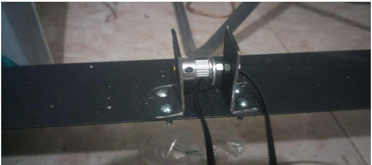
Figure 5.16: Timing Pulley installation
