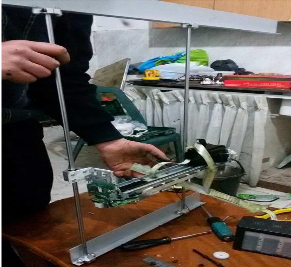
Figure 5.6: Linear guide motion and Y-axis installation
