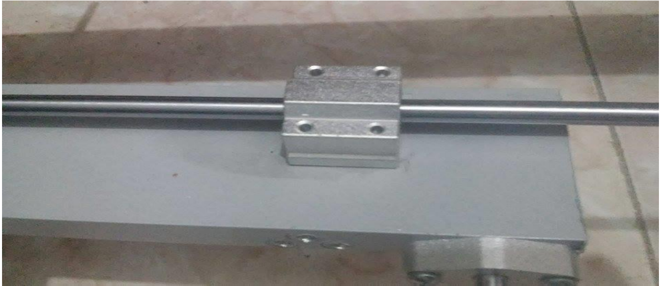
Figure 5.13: Linear bearing motion Installation
