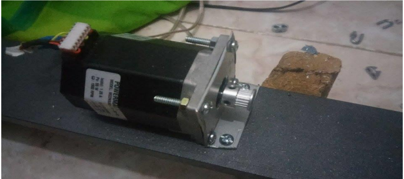
Figure 5.15: X-axis Stepper motor installation
